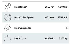
\*Performance data based on a standard day with zero wind. Field performance assumes a level, dry, paved runway, sea level at MTOW. Range based on a ferry mission at LRC with NBAA IFR reserves (100 nm alternate).
