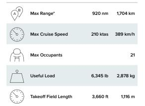
\*Performance data based on a standard day with zero wind. Field performance assumes a level, dry, paved runway, sea level at MTOW. Range based on a ferry mission, LRC at 10,000 feet with NBAA IFR reserves (100 nm alternate).
